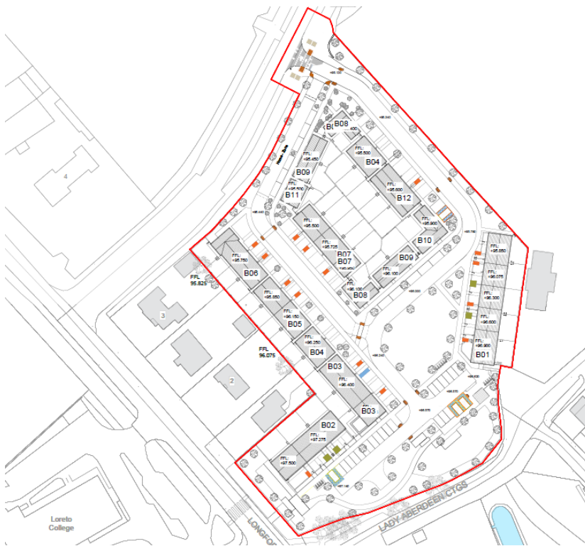
Figure 4: Site layout plan showing bin storage areas highlighted in orange
